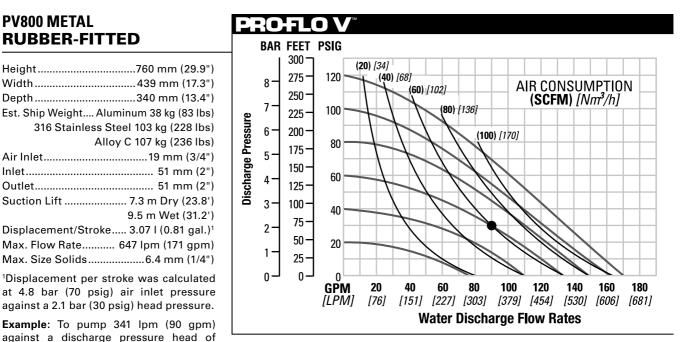
Flow rates indicated on chart were determined by pumping water.
