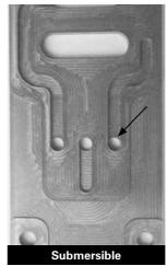
Next, install an optional submersible air valve gasket (04-2621-52). The submersible air valve gasket can be purchased as a spare part or included with the purchase of a new Pro-Flo  $V^{\text{TM}}$  pump.
