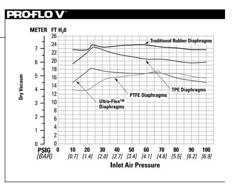
Suction lift curves are calibrated for pumps operating at 305 m (1,000') above sea level. This chart is meant to be a guide only. There are many variables which can affect your pump's operating characteristics. The
