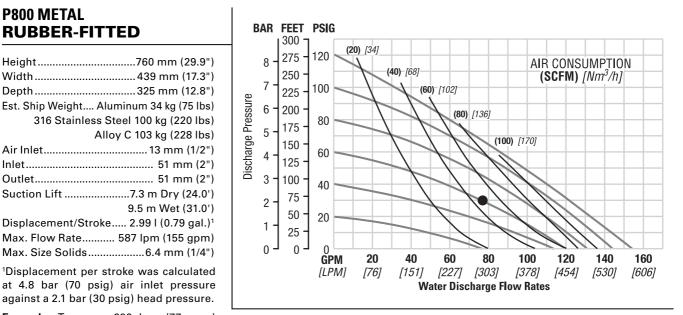
Flow rates indicated on chart were determined by pumping water.
