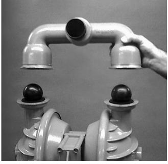
Step 3 Figure 3 Remove the discharge manifold to expose the valve balls and seats. Inspect ball cage area of manifold for excessive wear or damage. (*Figure 3*)
