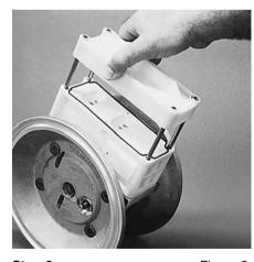
Step 2Figure 2Remove muffler plate and air valve boltsfrom air valve assembly (Figure 2)exposing muffler gasket for inspection.Replace if necessary.
