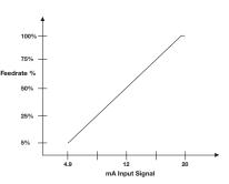
After a suitable amount of time dosing, verify your application with test equipment. Perform final adjustments to the metering pump setting (Variable Speed Mode) or Controller (4-20 mA input adjustments) to provide the required residual or results as determined through adequate test equipment or analysis.
