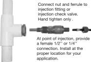
To prevent leaks, all the ferrules must be installed as illustrated.
