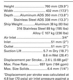
**Example**: To pump 481 lpm (127 gpm) against a discharge head of 1.4 bar (20 psig) requires 5.5 bar (80 psig) and 119
