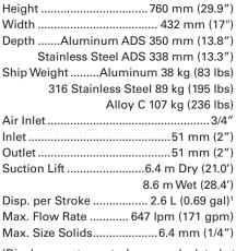
Displacement per stroke was calculated at 4.8 bar (70 psig) air inlet pressure against a 2.1 bar (30 psig) head pressure.
