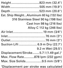
at 4.8 bar (70 psig) air inlet pressure against a 2.1 bar (30 psig) head pressure.
