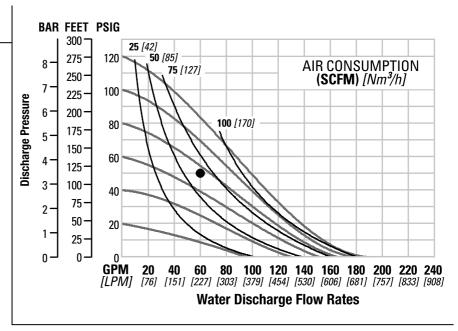
Flow rates indicated on chart were determined by pumping water with a vertically mounted, center ported ball check configuration. For optimum life and performance, pumps should be specified so that daily operation parameters will fall in the center of the pump performance curve.
