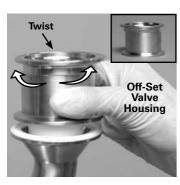
**NOTE**: To ensure proper alignment during reassembly of manifold/liquid chamber interface, turn off-set portion of valve housing to the left or to the right. This procedure works for the inlet manifold and discharge manifold connections.
