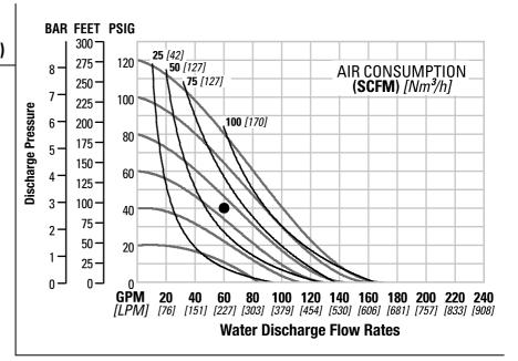
Flow rates indicated on chart were determined by pumping water with a vertically mounted, center ported ball check configuration. When alternate check valve options are used, multiply flow rate by appropriate factor. Mushroom check valve = 88%. For optimum life and performance, pumps should be specified so that daily operation parameters will fall in the center of the pump performance curve.
