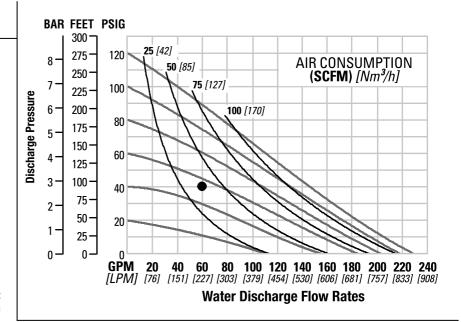
Flow rates indicated on chart were determined by pumping water with a vertically mounted, center ported ball check configuration. When alternate check valve options are used, multiply flow rate by appropriate factor. Flap check valve = 86%. For optimum life and performance, pumps should be specified so that daily operation parameters will fall in the center of the pump performance curve.
