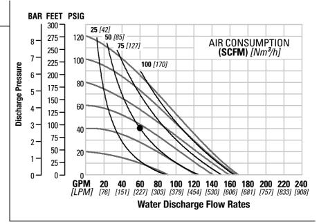
Flow rates indicated on chart were determined by pumping water with a vertically mounted, center ported ball check configuration. For optimum life and performance, pumps should be specified so that daily operation parameters will fall in the center of the pump performance curve.
