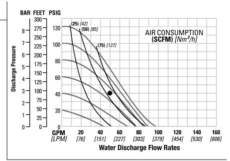
Flow rates indicated on chart were determined by pumping water with a vertically mounted, center ported ball check configuration. When alternate check valve options are used, multiply flow rate by appropriate factor. For optimum life and performance, pumps should be specified so that daily operation parameters will fall in the center of the pump curve.
