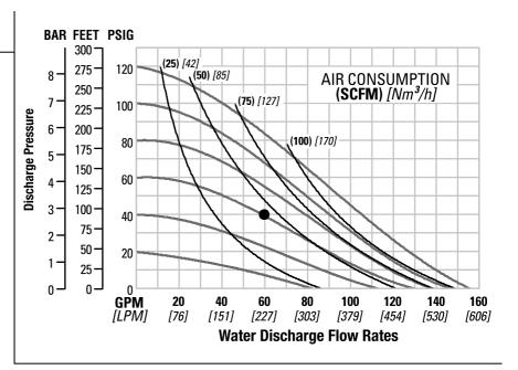
Flow rates indicated on chart were determined by pumping water with a vertically mounted, center ported ball check configuration. When alternate check valve options are used, multiply flow rate by appropriate factor. Flap check valve = 83%. For optimum life and performance, pumps should be specified so that daily operation parameters will fall in the center of the pump curve.
