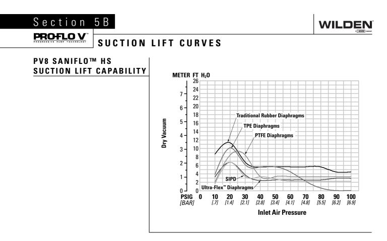
Suction lift curves are calibrated for pumps operating at 305 m (1,000') above sea level. This chart is meant to be a guide only. There are many variables which can affect your pump's operating characteristics. The number of intake and discharge elbows, viscosity of pumping fluid, elevation (atmospheric pressure) and pipe friction loss all affect the amount of suction lift your pump will attain.
