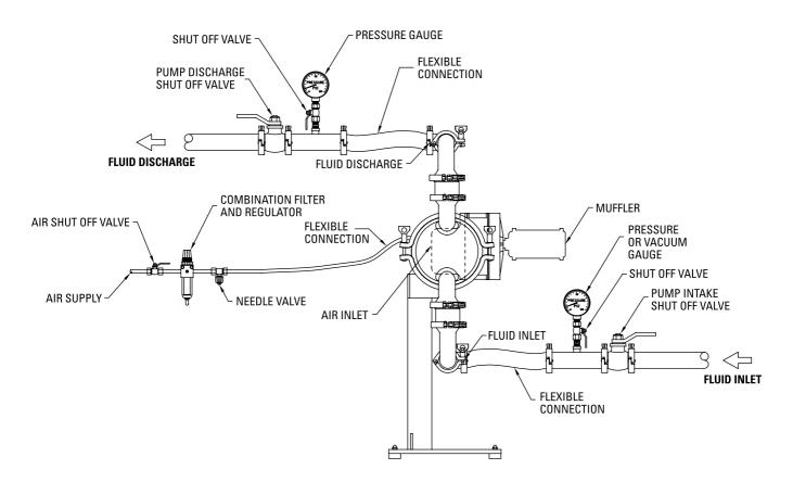
**NOTE:** In the event of a power failure, the air shut off valve should be closed, if restarting of the pump is not desirable once power is regained.
