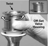
**NOTE:** To ensure proper alignment during reassembly of manifold/liquid chamber interface, turn off-set portion of valve housing to the left or to the right. This procedure works for the inlet manifold and discharge manifold connections.
