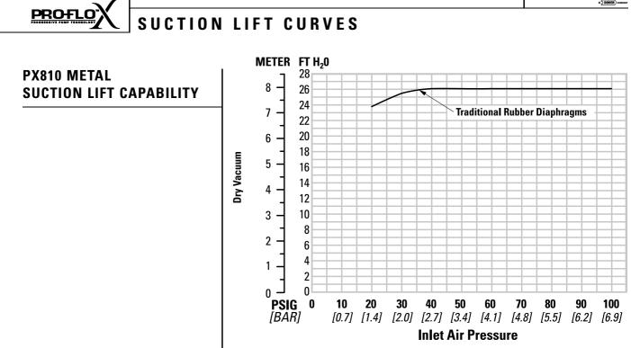
Suction lift curves are calibrated for pumps operating at 305 m (1,000') above sea level. This chart is meant to be a guide only. There are many variables which can affect your pump's operating characteristics. The
