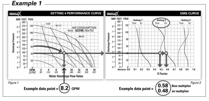
This is an example showing how to determine flow rate and air consumption for your Pro-Flo  $X^{\text{TM}}$  pump using the Efficiency Management System (EMS) curve and the performance curve. For this example we will be using 4.1 bar (60 psig) inlet air pressure and 2.8 bar (40 psig) discharge pressure and EMS setting 2.
