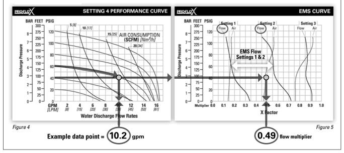
This is an example showing how to determine the inlet air pressure and the EMS setting for your Pro-Flo X<sup>™</sup> pump to optimize the pump for a specific application. For this example we will be using an application requirement of 18.9 lpm (5 gpm) flow rate against 2.8 bar (40 psig) discharge pressure. This example will illustrate how to calculate the air consumption that could be expected at this operational point.
