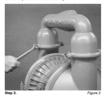
Utilizing the 11/16" box wrench, remove the two small clamp bands that fasten the discharge manifold to the liquid chambers.
