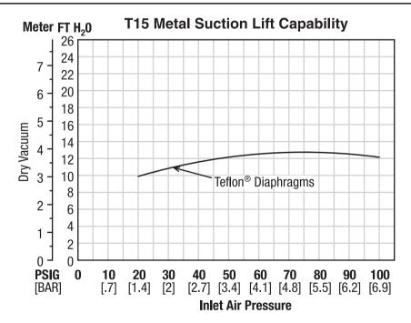
Suction lift curves are calibrated for pumps operating at 305 m (1,000') above sea level. This chart is meant to be a guide only. There are many variables which can affect your pump's operating characteristics. The number of intake and
