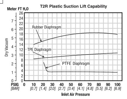
Suction lift curves are calibrated for pumps operating at 1,000' (305 m) above sea level. This chart is meant to be a guide only. There are many variables which can affect your pump's operating characteristics. The number of intake
