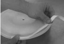
Starting at any point, place the PTFE The ends of the tape should overlap tape directly on top of the diaphragm bead. Press lightly on the tape to ensure that the adhesive holds it in place during assembly. Do not stretch the tape during placement on the diaphragm.
