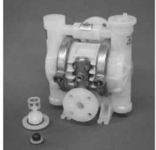
Remove the top liquid retainer and retainer o-rings, discharge valve balls, seats and valve seat o-rings from the liquid chamber and inspect for nicks, gouges, chemical attack or abrasive
