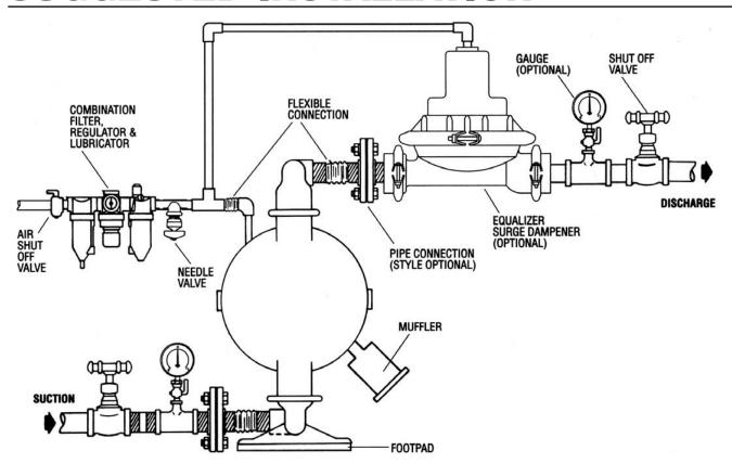
**AIR-OPERATED PUMPS:** To stop the pump from operating in an emergency situation, simply close the shut-off valve (user supplied) installed in the air supply line. A properly functioning valve will stop the air supply to the pump, therefore stopping output. This shut-off valve should be located far enough away from the pumping equipment such that it can be reached safely in an emergency situation.
