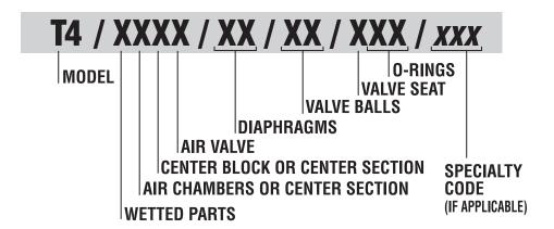
In the case where a center section is used instead of a center block and air chambers, the designation will be as follows: Aluminum = AA, Polypropylene = PP
