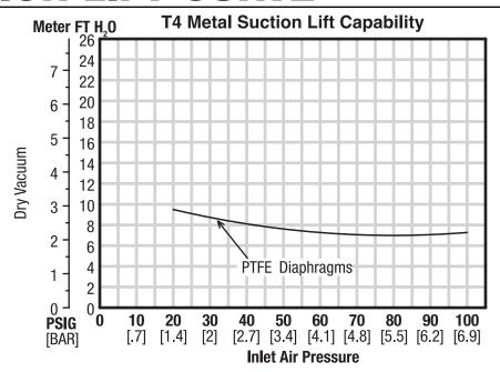
Suction lift curves are calibrated for pumps operating at 1,000' (305 m) above sea level. This chart is meant to be a guide only. There are many variables which can affect your pump's operating characteristics. The number of intake and discharge
