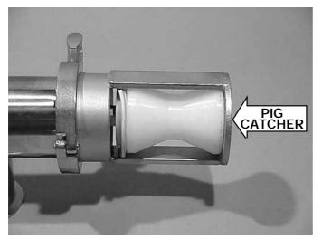
After securing tee section cap with clamp band, install pipe pig catcher to end of process discharge piping. When installation of pipe pig catcher is complete, begin purging process by continually pressing the system purge button on right side of control panel. When purging process is complete, retrieve pipe pig from pipe pig catcher. *(Figure 4)*
