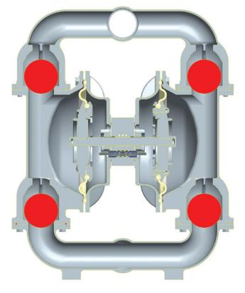
A cross section of the Wilden<sup>®</sup> Advanced<sup>™</sup> Series 3-inch stainless steel "drop-in" wetted path. It features a larger cross sectional area (compared to a traditional 3-inch stainless-steel wetted path) to reduce internal friction losses.
