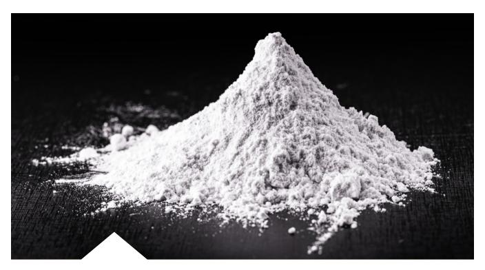
Though titanium dioxide (TiO<sub>2</sub>) may appear to be a fine powder, in reality it is very abrasive in slurry form, which is its general state when used in paint and coatings production. Therefore, when AODD pumps are used in its transfer, the diaphragms must be able to withstand outer-piston abrasion, the chance of which the innovative integral piston design of the Wilden® Chem-Fuse Diaphragm eliminates.
