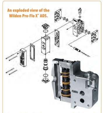
Few pump developers have taken a more proactive approach to the design and performance of the pump's Air Distribution System (ADS) than Wilden. With its Pro-Flo X<sup>™</sup> ADS (pictured), Wilden allows operators to set its pumps to the most efficient level for optimum flow and energy efficiency.
