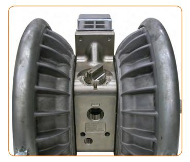
Wilden's Pro-Flo X<sup>™</sup> air distribution system (ADS) provides top-of-the-line operational flexibility through its patented Efficiency Management System (EMS<sup>™</sup>) that allows the user to optimize the ADS for any application demands regardless of pump size through the use of a control dial that allows the user to select the flow rate that best suits the application.
